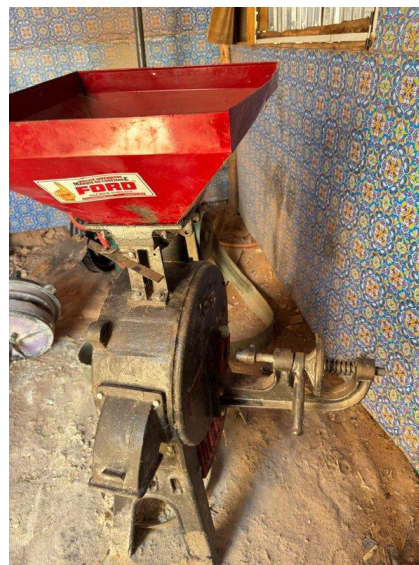
Figure 2: Grain feeding hopper and grinding assembly
