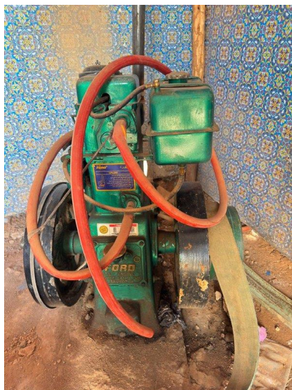
Figure 1: Diesel engine and belt-driven grinding unit
